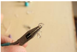
Hold Chain with Flat nose pliers and open where the break is.
